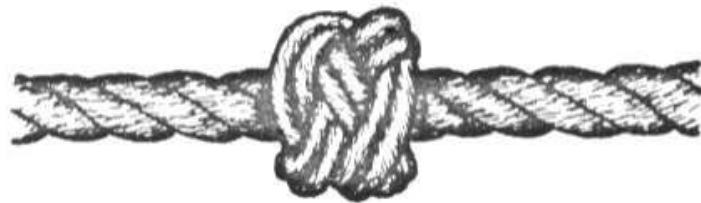
Fig. 23. – A shroud knot (fourth variation).
